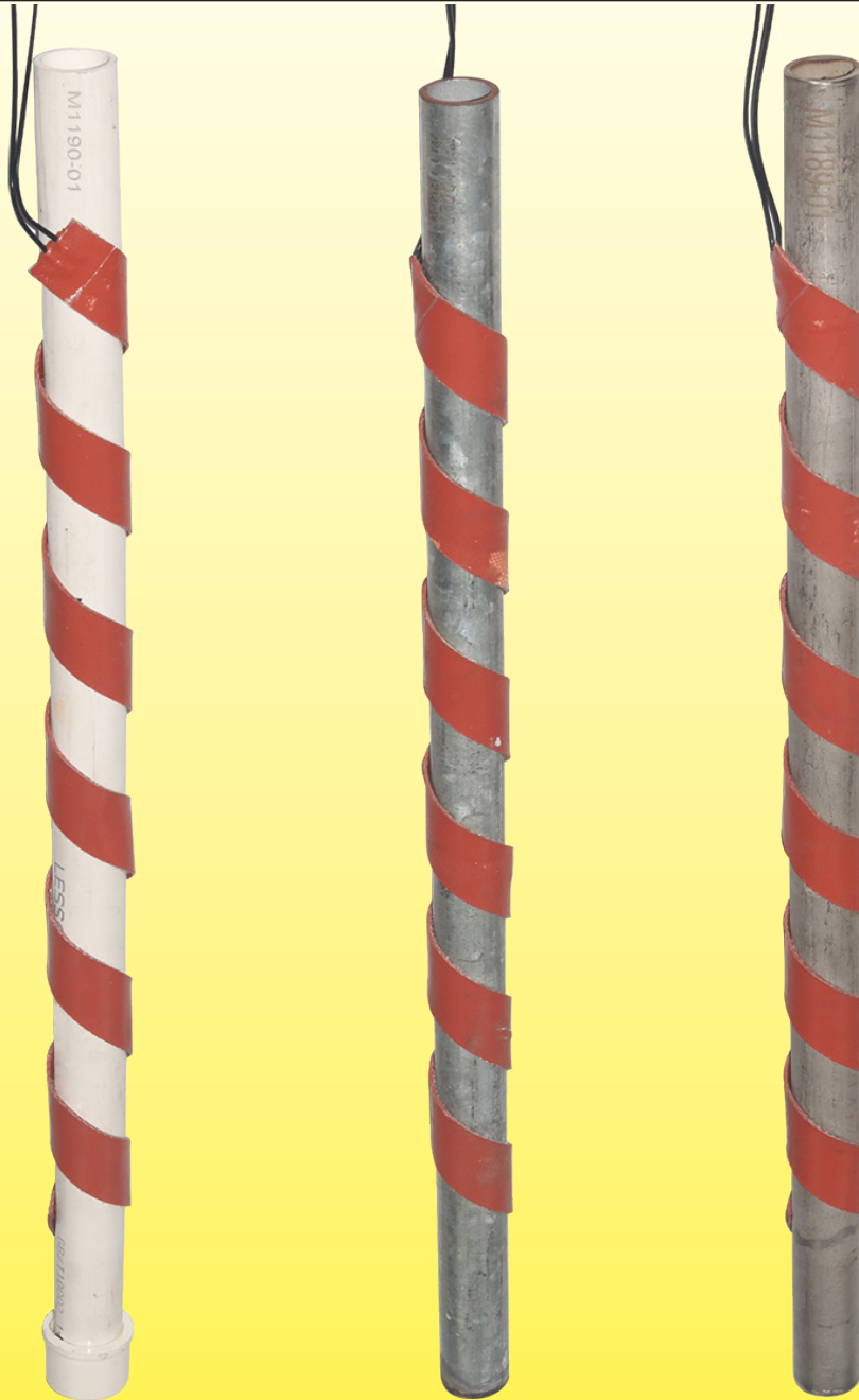
Condition of the comparative tests: Silicone heating ribbons wound on tubes of external diameter 25mm, in PVC-U, galvanized steel and stainless steel
